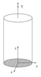
Determine the strain field in the rod by using the relations as follows:
